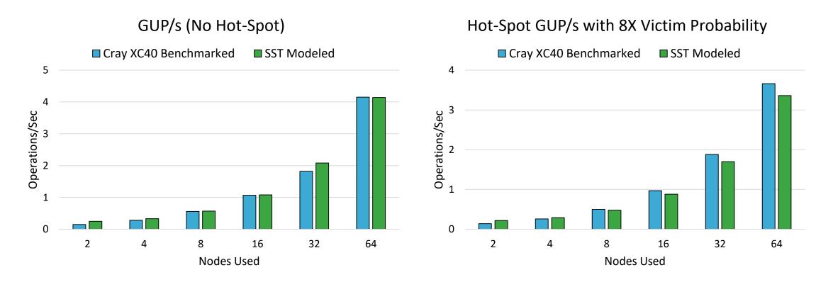
Compare Cray XC40 (Blue) to SST (Green), results are for 32 PEs per node. With no hot-spot, the GUP/s results show strong correlation with typically low (10-15%) predictive error. With an 8X increase in probability of selecting a victim node, predictive accuracy decreases at scale (still around 10-15%)
