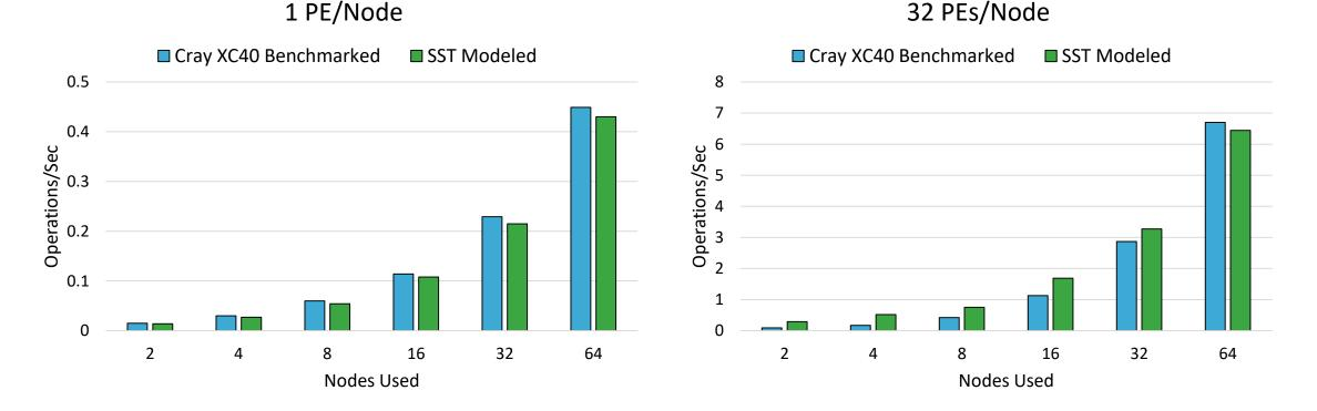
Compare Cray XC40 (Blue) to SST (Green) – strong qualitative trend. Predictive error is approx. 10% for 1 PE/node but up to 200% for very small node counts when using 32PE/node.
