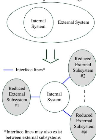
Fig. 1. Modeling of an interconnected power system for real-time study
