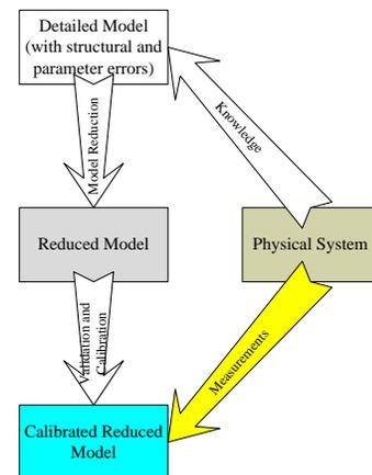
Fig. 2. Process to calibrate reduced models for external power systems
