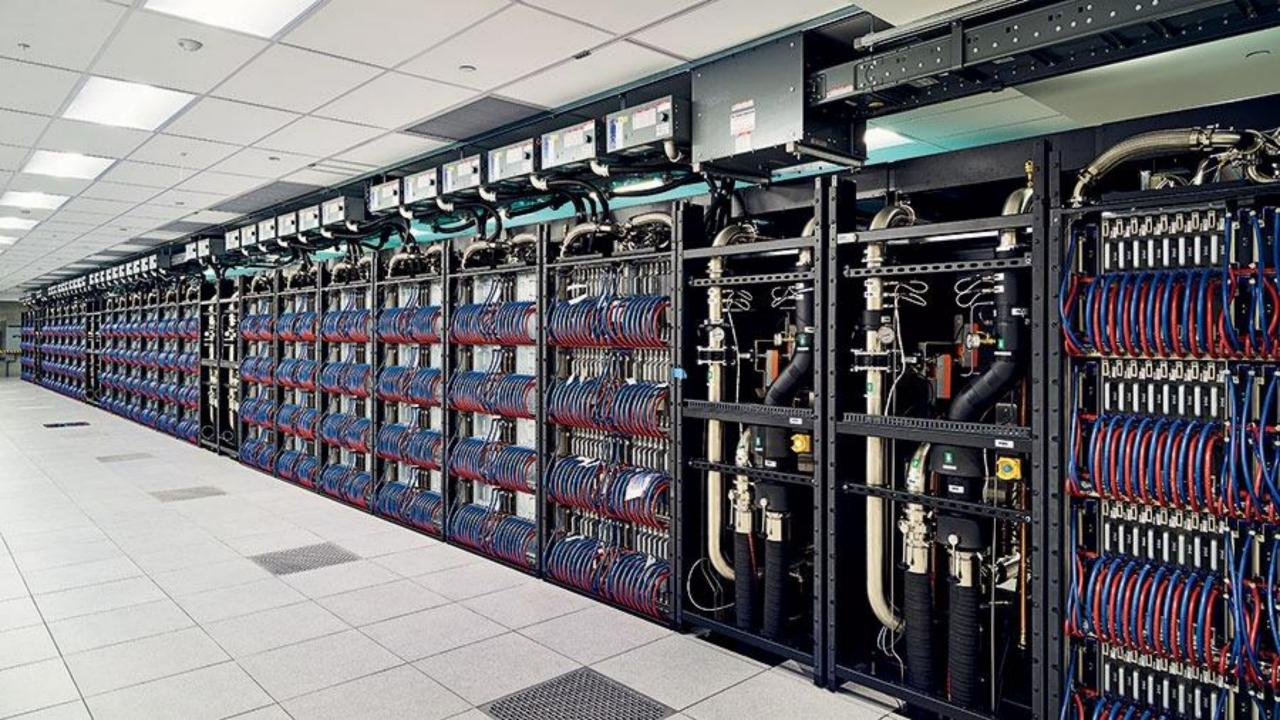
Aurora is: 166 Racks 10,624 Nodes 21,248 CPUs 63,744 GPUs 84,992 NICs 8 PB HBM 10 PB DDR5
