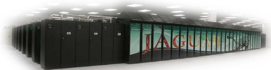
**Titan** will be an upgrade to Jaguar in late 2012. Titan will add next generation NVIDIA GPUs to the nodes of Jaguar resulting in a system with a peak performance of between 10 and 20 PF. The Spider disk subsystem will be upgraded to provide up to 1 TB/s of disk bandwidth and up to 30 PB of storage.
