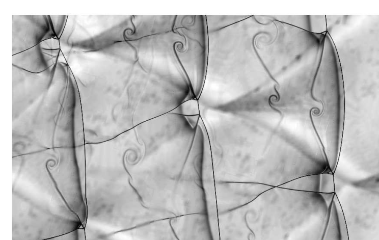
Top: Front on triple point tracks after the bend for \alpha = 15 (shown rotated). Right, top: Strengthening of DMR pattern (open triangles) under expansion at 130 \mu s and 140 \mu s simulated time. Right, bottom: Weakening TMR in over-driven region (open squares) at 130 \mu s and 140 \mu s .
