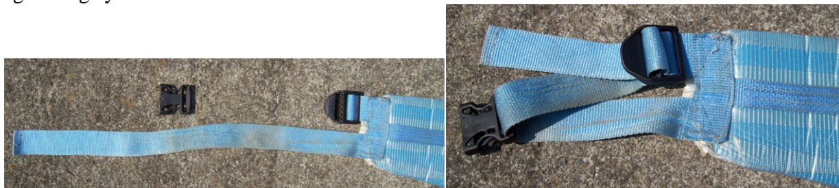
Waist strap construction showing the 4" base strap sewn to the tip of the hip belt.
