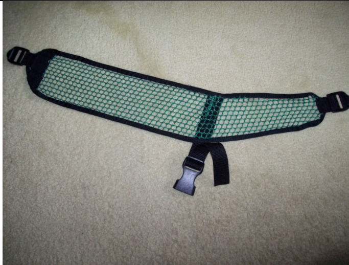
Figure 3. The hex mesh shoulder strap. The top of the strap is on the left. The strap is 3½” wide. Not counting the buckles it is 21” from the top to the bottom and the top of the chest strap is 12” from the top
