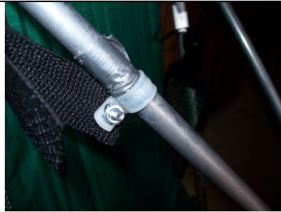
Figure 2b. Close-up of upper attachment showing 1" wide duct tape placed above clamp to prevent sliding up under load
