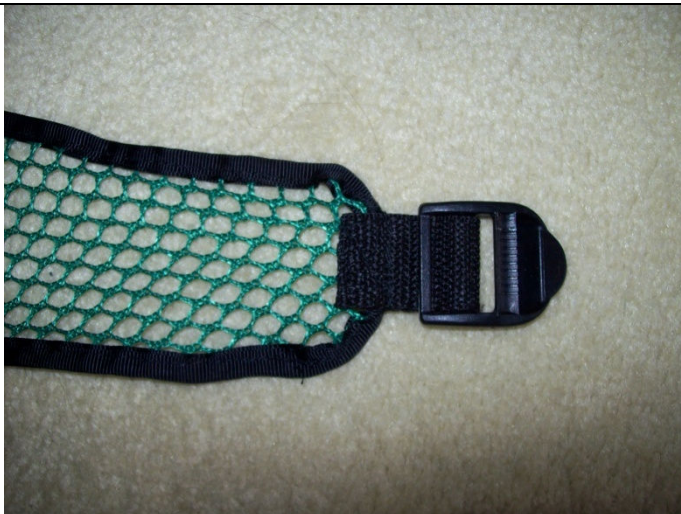
Figure 6. Bottom slide adjuster is sewn on top of the mesh. Be sure that both the ribbon and the mesh have several sewing seams run back and forth over them. (Same is true for the top slide adjuster.)
