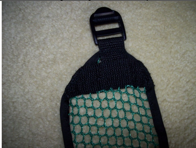
Figure 5 The header is the key design feature that makes the mesh strap work. 1" polypropylene is sewn to both sides of the mesh and a stiff steel shim is slipped into the pocket formed before the edge is sewn shut. This holds the mesh flat and wide under load.
