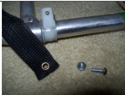
Figure 1b. shows grommet in strap and ½" #10 screw and nut
