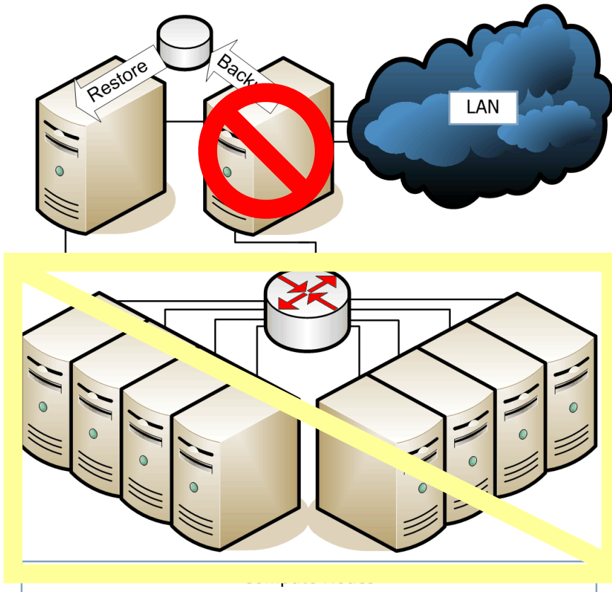
Active/Standby Head Nodes with Shared Storage
