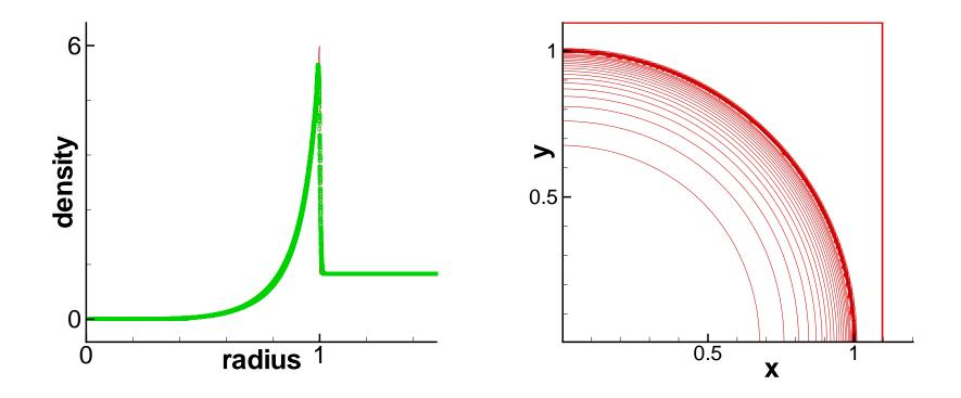
Figure 1: 2D Sedov blast, plot of density. T = 1. N = 160.  $\Delta x = \Delta y = \frac{1.1}{N}$ . TVB limiter parameters  $(M_1, M_2, M_3, M_4) = (8000, 16000, 16000, 8000)$ .
