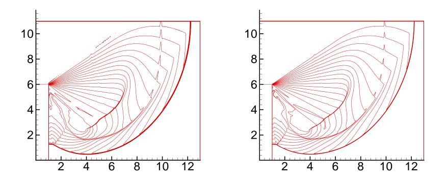
Figure 2: Shock diffraction problem. Density: 20 equally spaced contour lines from  $\rho = 0.066227$  to  $\rho = 7.0668$ . Left:  $\Delta x = \Delta y = 1/32$ ; Right:  $\Delta x = \Delta y = 1/64$ .
