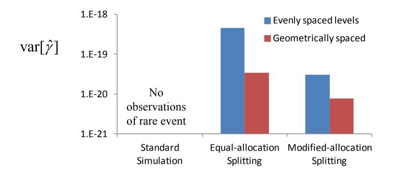
Prob. of advancing from level *j*-1 to *j* depends on starting state from level *j*-1 (modified allocation not necessarily optimal)
