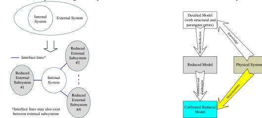
Fig. 1. Modeling of an interconnected power system for real-time study Fig. 2. Process to calibrate reduced models for external power systems
