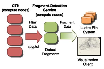
Fragment detection service provides on-the-fly data analysis with no modifications to CTH.
