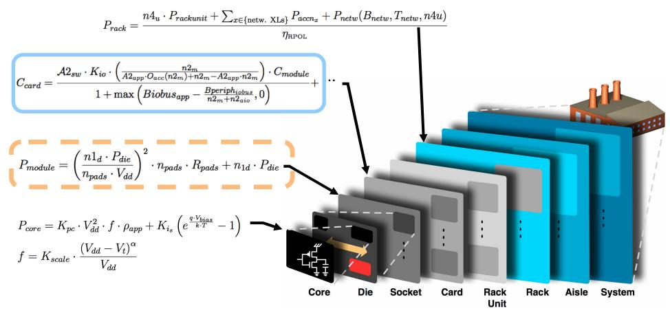
**Notation**: C<sub>xx</sub>: computation throughput (FLOPS) P<sub>xx</sub>: Power; f: clock frequency; K<sub>xx</sub>: constant; V<sub>xx</sub>: voltage; R<sub>xx</sub>: resistance;
