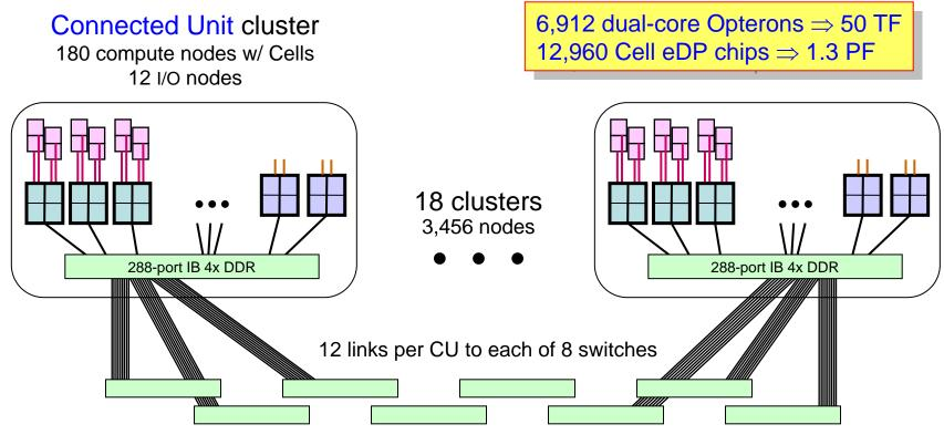
Eight 2<sup>nd</sup>-stage 288-port IB 4X DDR switches
