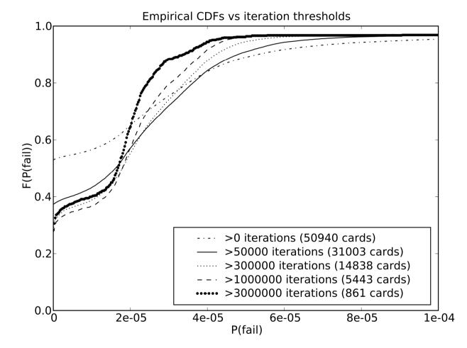
Population of failing cards has a mode around  $P_f = 2x10^{-5} = ^4$  failures/week
