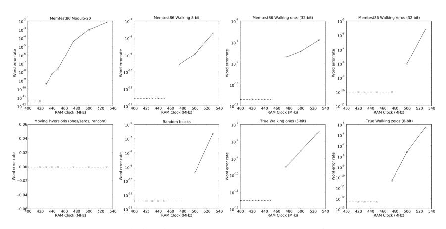
Positive control displays pattern sensitivity of memory tests
