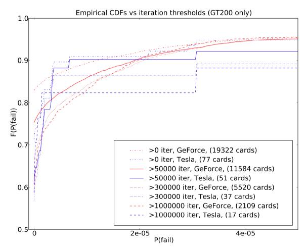
Tesla traces are rougher from poorer sampling, but appear to represent same error distribution as GeForce data.
